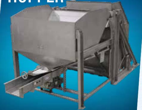
Hoppers for bulk loading while regulating the discharge of product by using an adjustable slide gate and vibratory conveyor.
