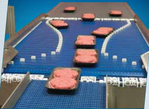
AIM Technology by Intralox® is designed specifically to perform in washdown environments and optimized for cleaning and sanitation processes.
