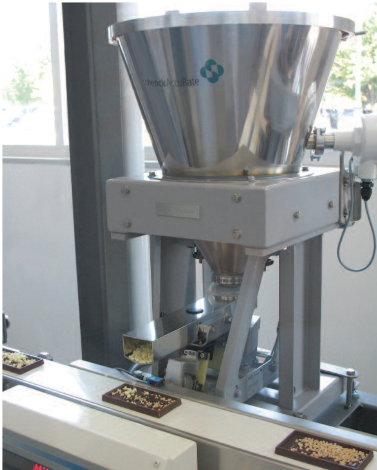
A vibratory feeder accurately dispenses an ingredient into a chocolate base bar's recessed cavity.
